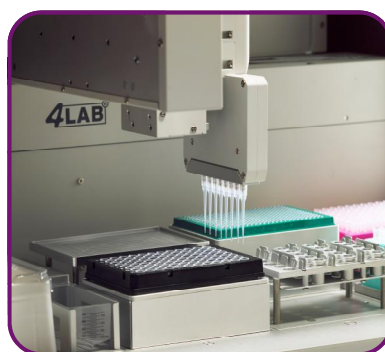
Figure 3: The NeodymlronBor magnetic separation plate used by 4LAB for PCR product clean-up and dye terminator removal.
